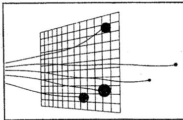
Filters that operate through the interception mechanism may employ widely spaced or densely packed filter media, depending upon requirements. Coarser filters will intercept larger particles. More densely packed filters will intercept smaller particles, but will also restrict the airflow, posing the problem of high-pressure drop. Increasing the filter area can compensate for high-pressure drop, but a balance must be achieved between filter area and practical physical limitations.
